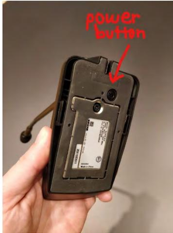
Press and Hold the **Power button** down for a few seconds (**colour ring will turn green when connected**).
