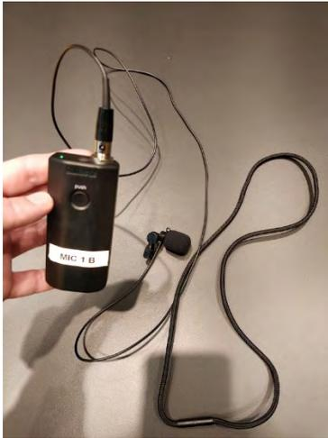
Press the PUSH button (**green light when connected**).
